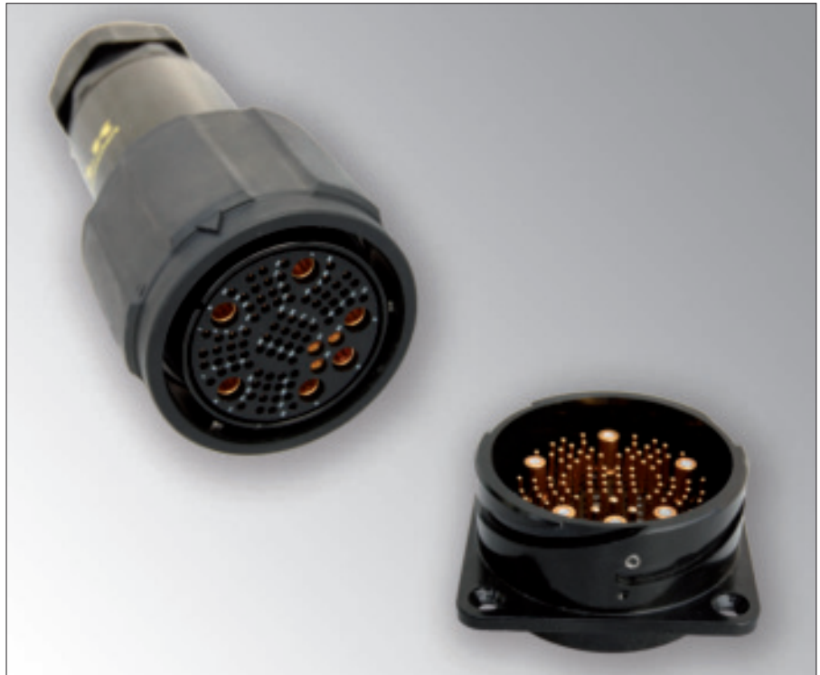
The LKA 40/89 connector is the largest in the coax series and it features 80 pins size 18 for signal transmission, 6 coaxial pins and 3 pins size 12 for power.
